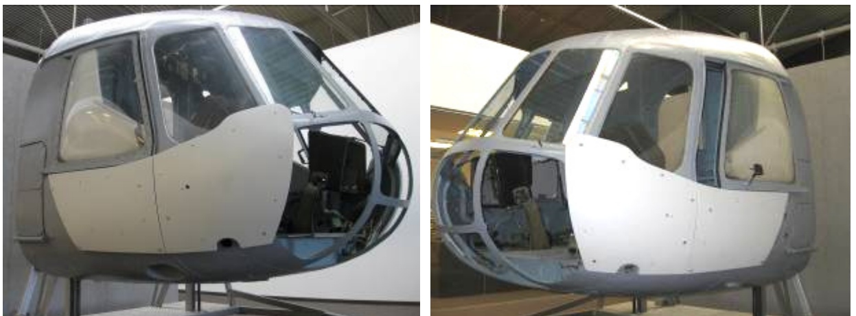
Fig.2 Outside ceramic composite panels installed
