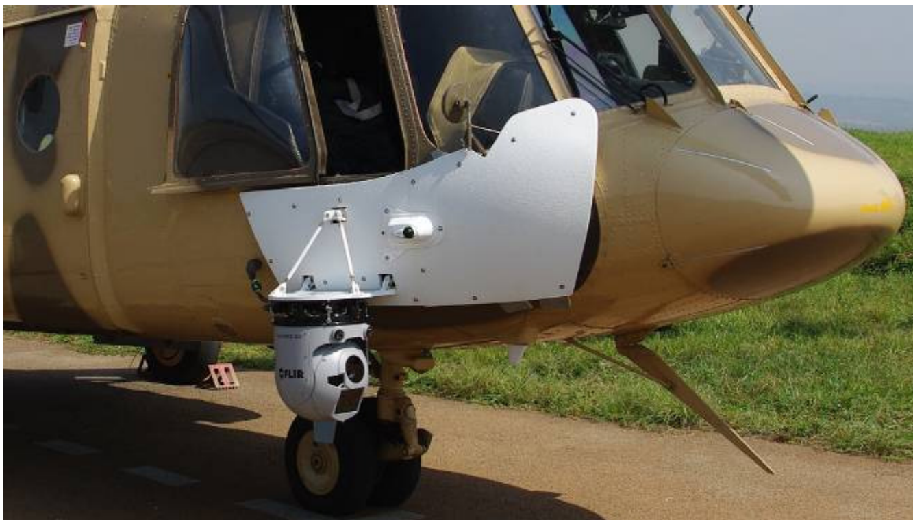
Fig. 8 Ceramic composite armor panel reworked for the installation of FLIR camera
